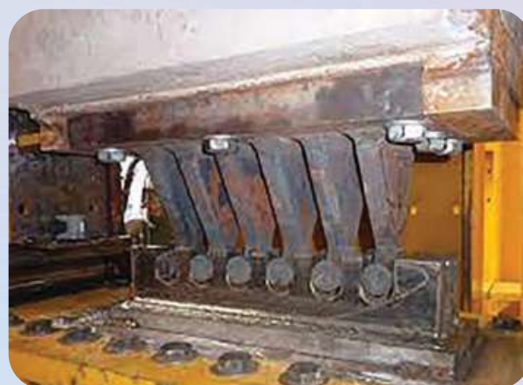
Photo 7. TADAS devices installed in the test machine.
