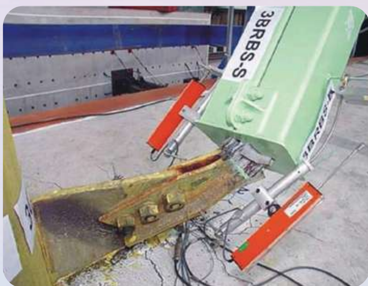
Photo 3. Out-of-plane buckling of the gusset plate of the BRB connection
