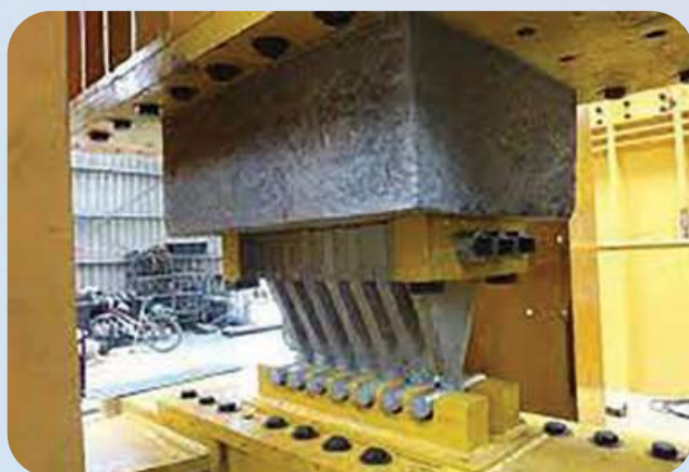
Photo 7. TADAS devices installed in the test machine.
